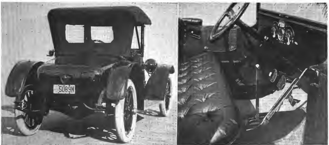
Left—Rear view of new Hupmobile roadster, showing tail light and license bracket mounted in the center. Right—Dash view, showing instrument board. Left—Lighting switch; center, speedometer; right, starting and ignition switch. All switches are controlled by Yale lock. Note pads on pedals
